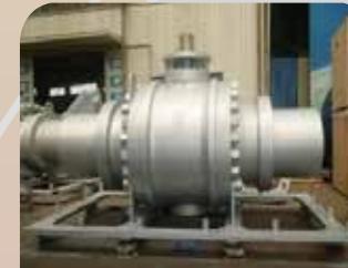
API 6D ASTM A216 WCB full bore trunion mounted ball valves, butt welded, welded ends, covered with 600mm pups API5L X60 12.7mm wall thickness, stainless steel 316L stem and seat.
