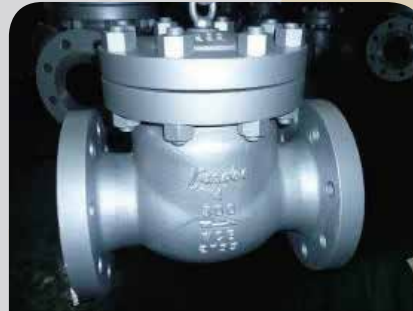
ASTM A216 Swing Check Valves, 4 Inch (DN100), 300LB (PN50), Flanged RF End, Full Bore, BS 1868, 13% CR Trim.
