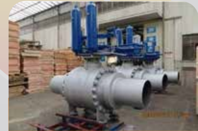
API 6D full bore trunion mounted ball valves, butt welded, with gas over oil actuator with remote telemetry, covered with 600mm pups X60 12.7mm wall thickness.
